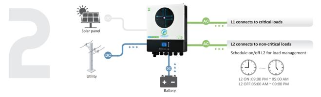
Only battery energy provides power to the loads.
